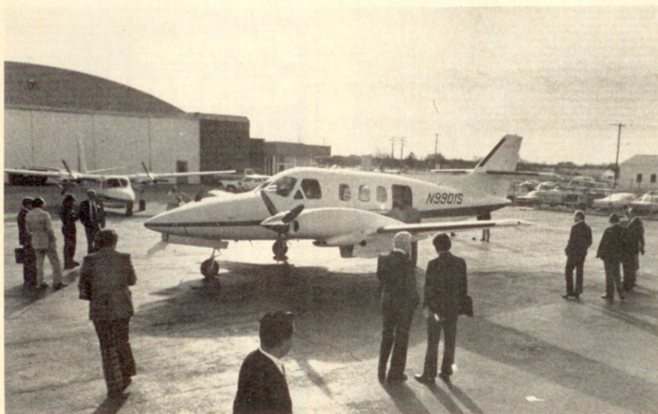
Low wing and mid-tail-mounted horizontal stabilizer separate new Rockwell Commander 700 from company's traditional high-wing twins. This pressurized, turbocharged model will roll off production lines next year, to be followed later by turboprop and jet versions.
